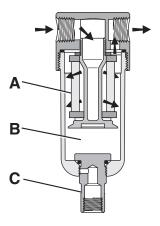
The contaminated air enters the element interior and is forced through a thick membrane (A) of "borosilicate" glass fibers coated with epoxy. Flow then passes through the element, and at this stage 99.97% of the sub micronic particles have been removed from the air stream. The tiny droplets coalesce together and are collected from the filter element by the outer drain layer.
